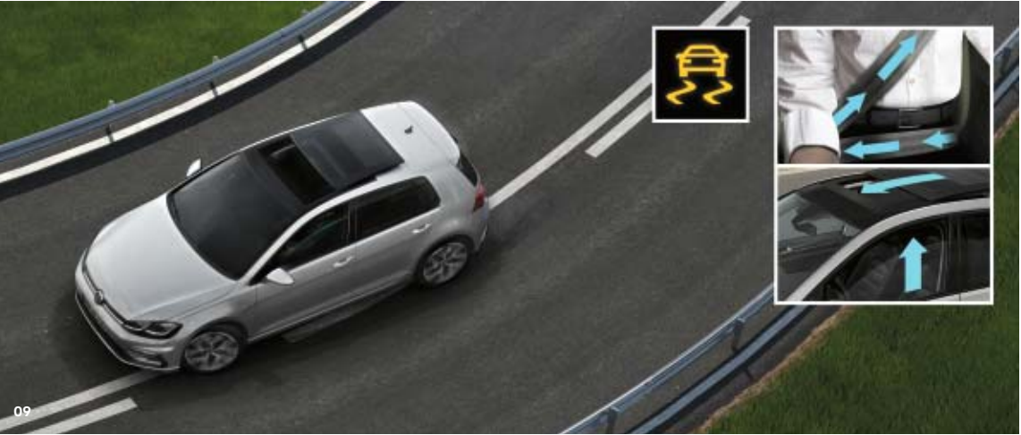
07 Using a camera installed behind the front windscreen, “Light Assist” main beam control detects oncoming traffic and vehicles driving ahead and automatically switches between main beam and dipped beam. SO
