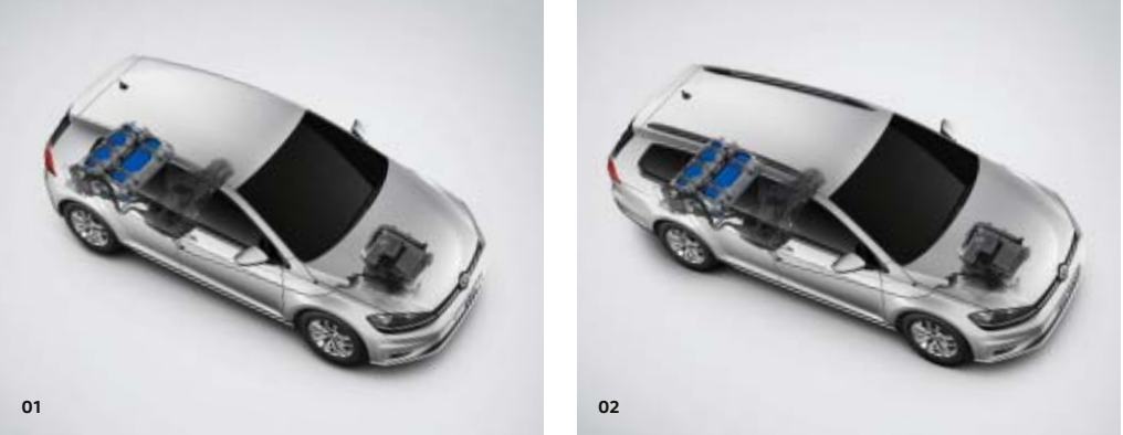
01| 02 The natural gas drive reduces consumption and has a positive effect on emissions. The natural gas tanks are hidden underneath the floor to save space so that they do not restrict the vehicle's flexibility or its storage space. And if the natural gas tank is empty, the additional petrol tank will easily take you to one of the 900 natural gas fuelling stations across Germany. SO
