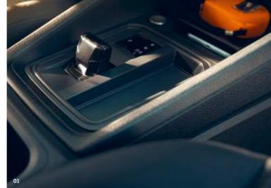
01 Dual-clutch gearbox (DSG).1), 2) No time for idling. The new Caddy Cargo can be equipped with a 7-speed dualclutch gearbox for fully automatic gear changes without any interruption in tractive force.
